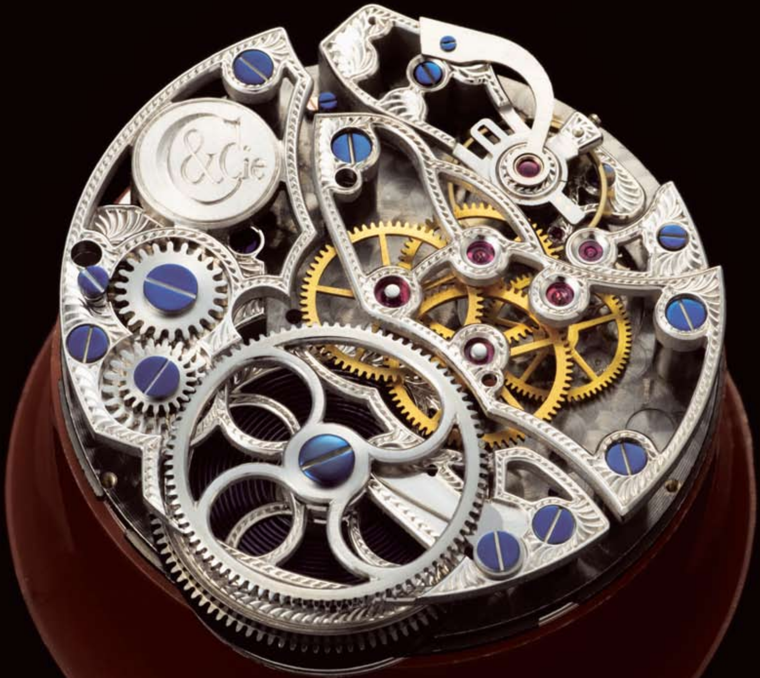
A. Schild Caliber 690 from 1935 looks nothing like it did before Kees Engelbarts got his hands on it.
